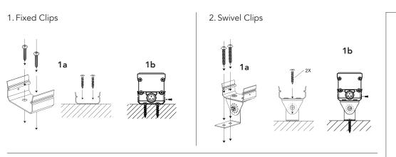
3.3" Arc and 6" Arc Bracket Installation
