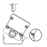
**2b** Fixture will pivot on notch as it is pushed down.
