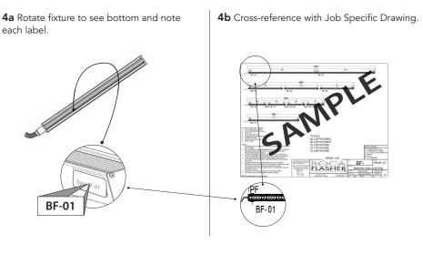
**IMPORTANT NOTE:** Not clicking fixtures together represents an incomplete install and voids the warranty. If any fixtures are damaged as a result of improper installation
