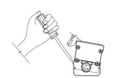
**8c** Once released from one notch, fixture can be fully removed.
